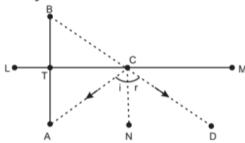
[Hint: CN is normal to the mirror, also, angle of incidence = angle of reflection].
